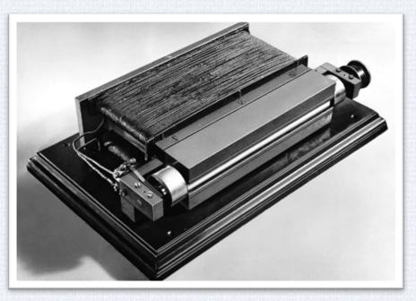
Prototype of a dynamo-machine invented by Werner von Siemens in 1966. Source:www.siemens.com/history/en/news/1051\_wern er\_von\_siemens.htm
